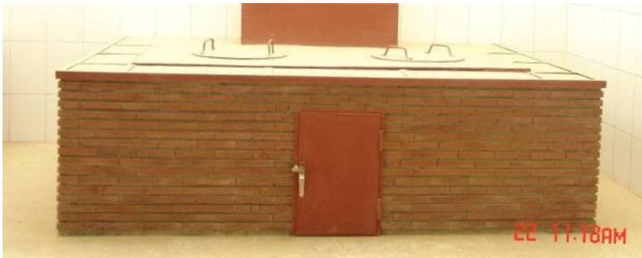
Figure 18 :New wood fired stove. Fire brick and steel construction with steel covers
