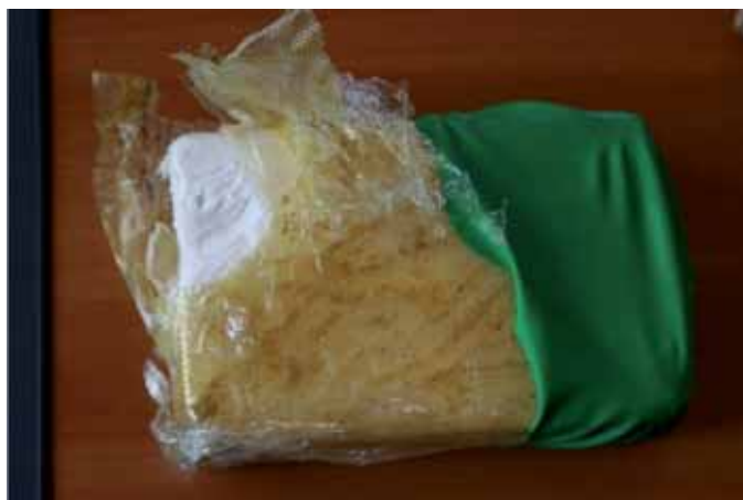
Under the transparent plastic bag each brick was wrapped in a balloon enhancing its water resistance.
