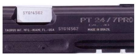
Figure V. Example of an alphanumeric marking on the barrel of a firearm
