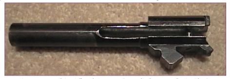
Figure I. A deactivated SIG Sauer P226 barrel demonstrating a slot cut into the feed ramp
